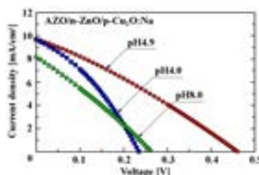
Figure 1: pH dependence of zinc acetate aqueous solution for J-V characteristics of AZO/n-ZnO/p-Cu<sub>2</sub>O: Na solar cells
