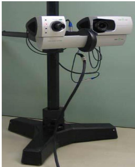
Fig. 6 - Steinbichler's 3D White Light Scanning Machine (COMET 5)
