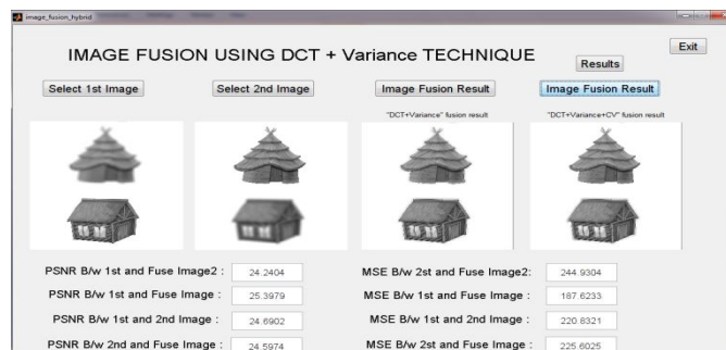
Fig. 11 showing the results of the DCT + variance based technique + CV based fusion
