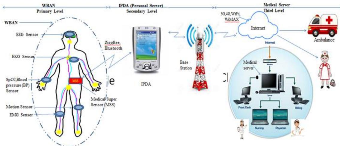
Figure 1. Three Level Architecture.
