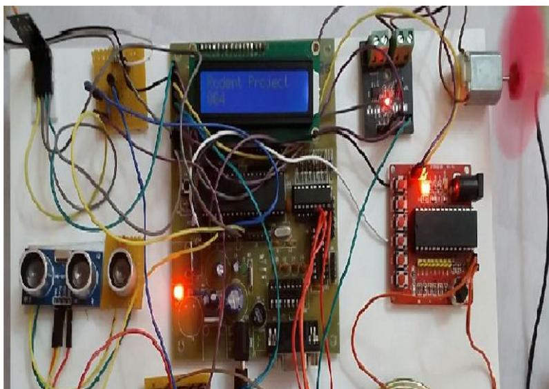
Figure 10:LCD displays the time interval between sounds
