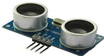
Figure 3: HC-SR04 Ultrasonic Sensor
