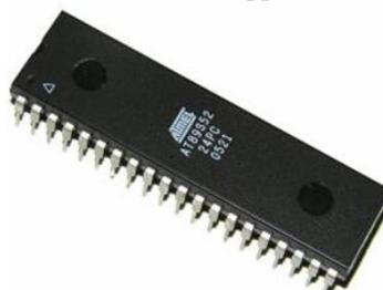
Figure 7: at89s52 Microcontroller
