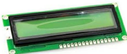
Figure 8: Hitachi hd44780 LCD controller with 16x2 compatible LCD screen
