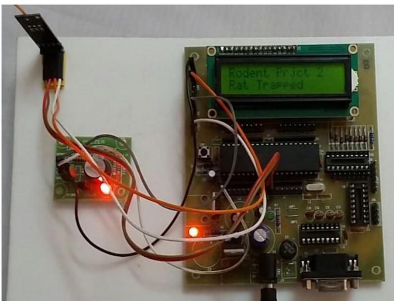
Figure 11:LCD displays “Rat Trapped” and buzzer is triggered
