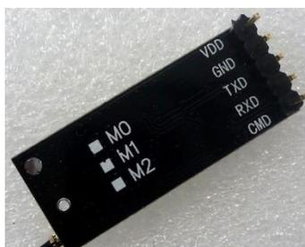
Figure 6: USB UART Serial port Wireless 2.4G Module replace Zigbee APC220 NRF24101 + CC1101
