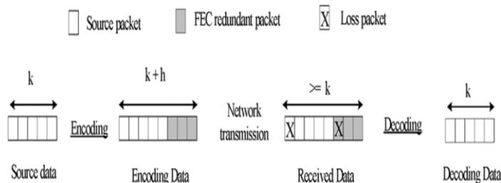
Fig. 2. FEC encoding and decoding.
