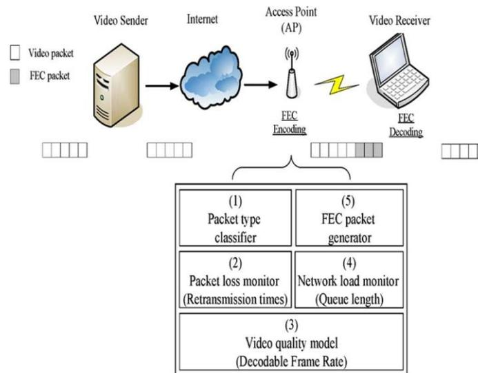
Fig. 5. Architecture of ERED-FEC controller
