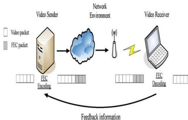
Fig. 3. Sender-based FEC scheme.
