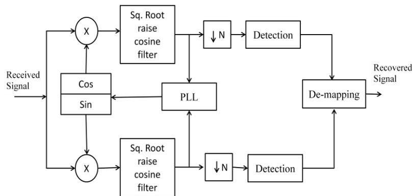
Fig. 4. Block diagram of QAM Demodulator
