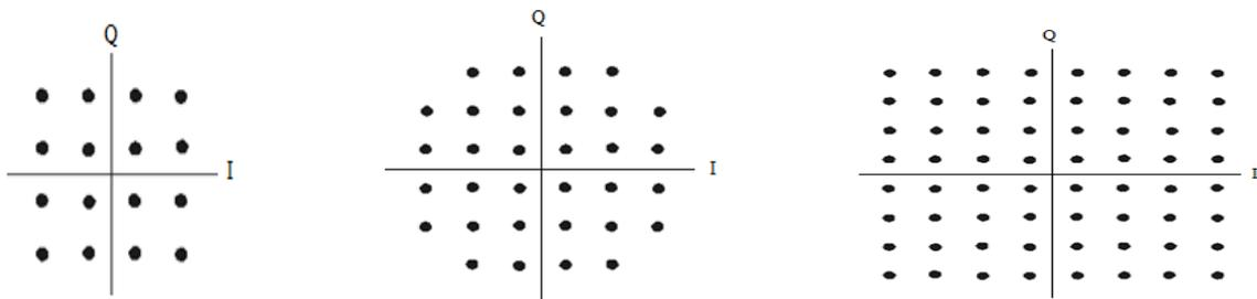
Fig. 3. Constellation diagrams of 16, 32, 64 QAM
