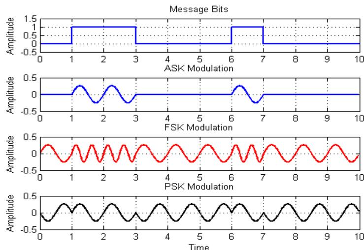
Fig. 1. Modulated signal waveforms of ASK, FSK and PSK [7].
