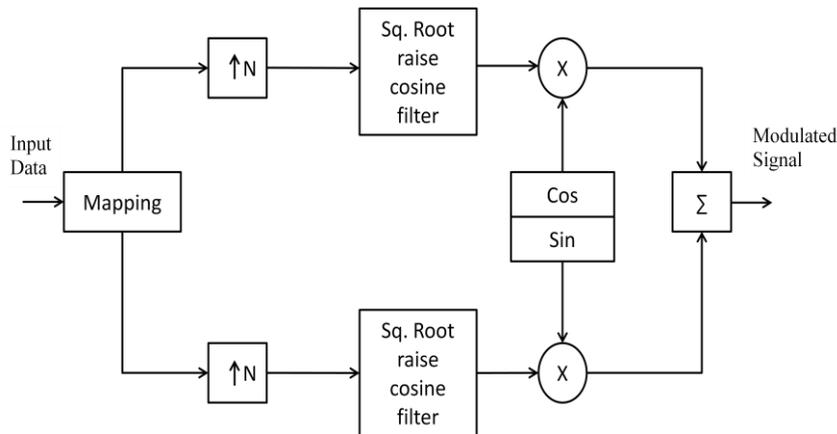
Fig. 2. Block diagram of QAM Modulator
