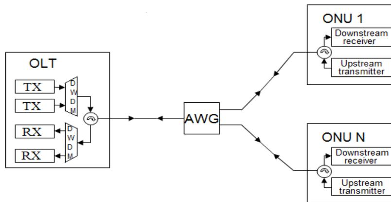
Fig.4. WDM-PON architecture
