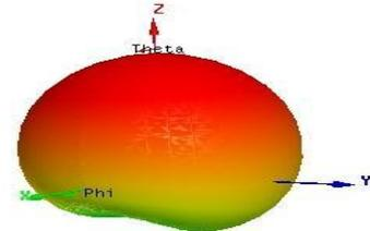
Fig 6.10:Gain of Rectangular microstrip antenna with parasitic patch on left side of radiating patch
