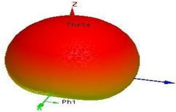
Fig 6.9:Gain of Rectangular microstrip antenna
