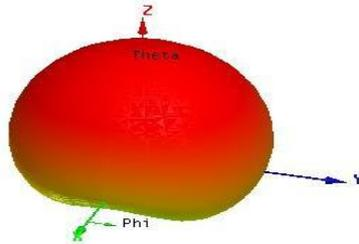
Fig 6.11:Gain of rectangular microstrip antenna using Parasitic patch on top side of radiating patch
