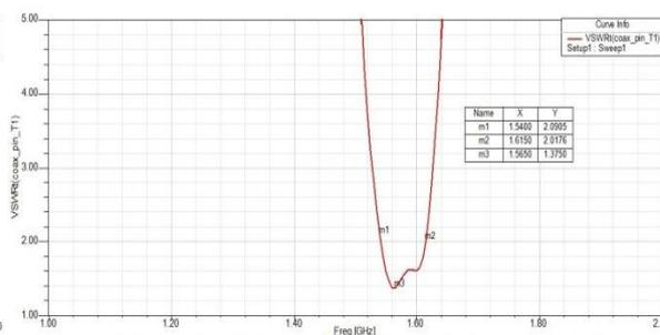
Fig 6.4: VSWR of rectangular microstrip antenna using parasitic patch on both side of radiating patch
