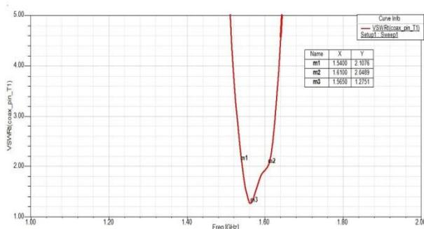
Fig 6.1: VSWR of Rectangular microstrip antenna
