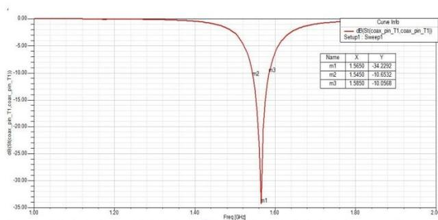
Fig 6.5: Return loss of Rectangular microstrip antenna
