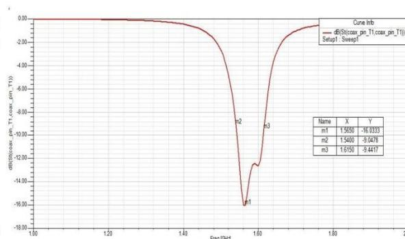
Fig 6.8: Return loss of rectangular microstrip antenna using parasitic patch on both side of radiating patch
