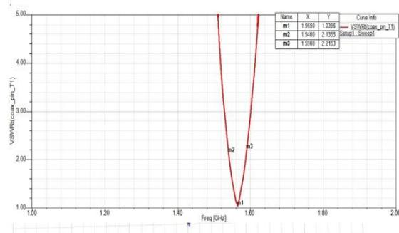
Fig 6.2: VSWR of Rectangular microstrip antenna with parasitic patch on left side of radiating patch
