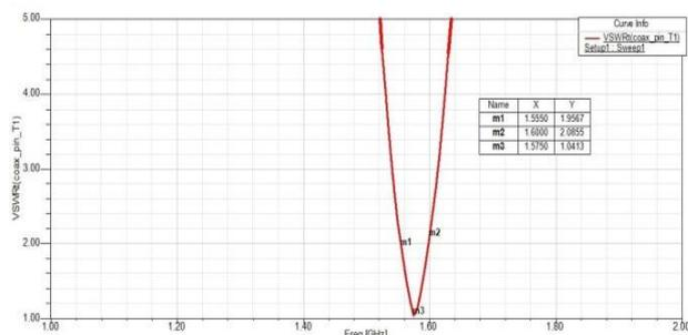
Fig 6.3: VSWR of rectangular microstrip antenna using Parasitic patch on top side of radiating patch
