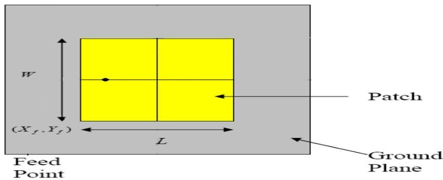
Figure 4.1: Rectangular microstrip antenna
