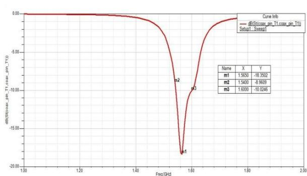
Fig 6.7: Return loss of rectangular microstrip antenna using Parasitic patch on top side of radiating patch
