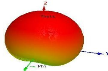
Fig 6.12: Gain of rectangular microstrip antenna using parasitic patch on both side of radiating patch
