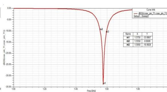
Fig 6.6: Return loss of Rectangular microstrip antenna with parasitic patch on left side of radiating patch
