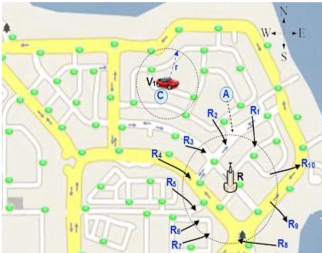
Fig.3.Example of an RSU choosing a road to send a packet to
