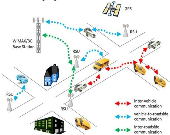
Fig 1.Simple Representation of RSU in VANET
