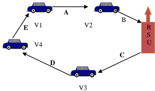
Fig 2. Sending a packet from a vehicle to an RSU
