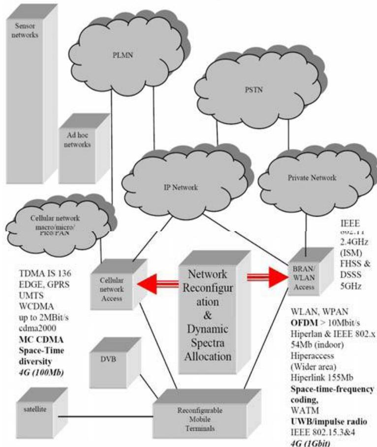
Fig.1: Composite radio environment in 4G networks
