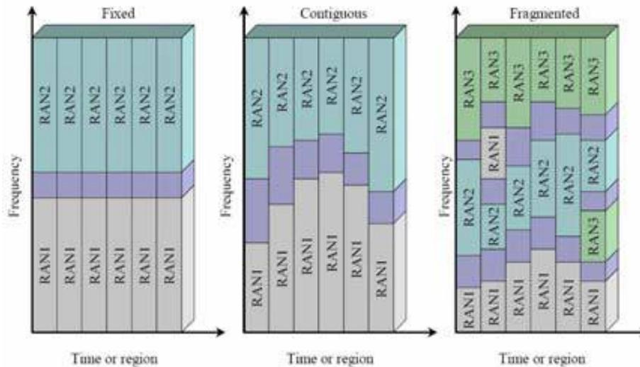
Fig .3 Fixed spectrum allocation compared to contiguous and fragmented DSA.
