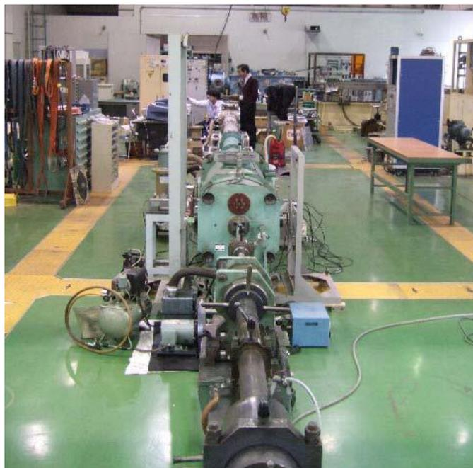
Fig. 2 Two stage light gas gun
