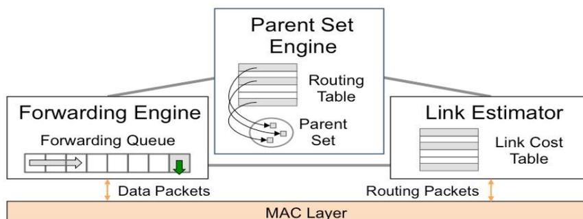
Fig.1. Main components of CTP+PPS.
