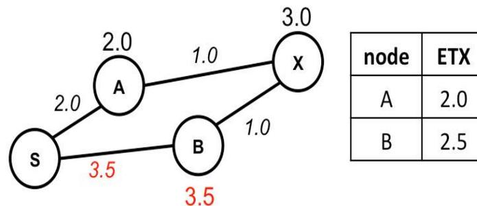
Fig.2. An example of a routing outley inconsistency in PPS without relaxing the loop-detection condition.
