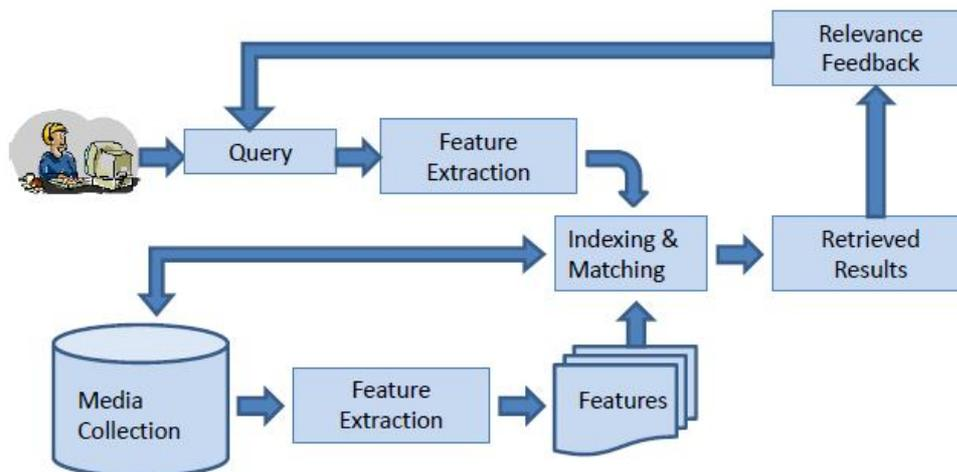
Figure1:- Block Schematic of Feature Extraction in Audio Visual Based Searching
