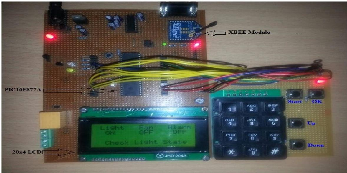
Figure 4: The control station (ADV user) made up of PIC16F877A and associated controls.
