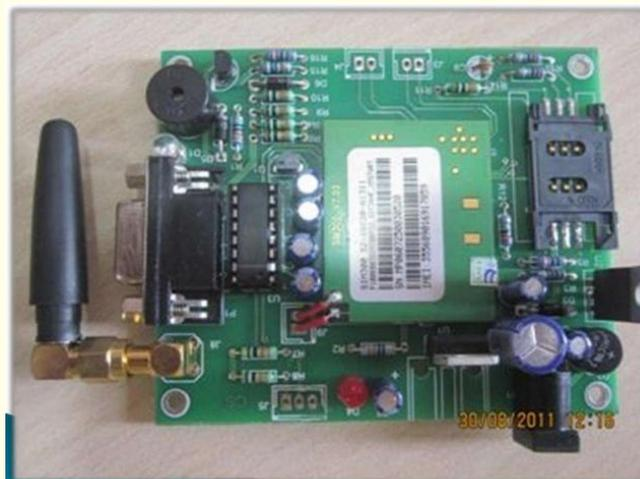
Fig 2 GSM Module
