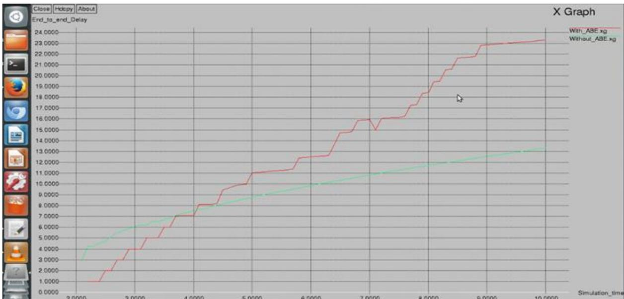
Fig.7 Graph showing End to end delay with ABE mechanism
