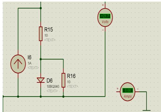
Figure 11: Open circuit voltage (21.7 V).
