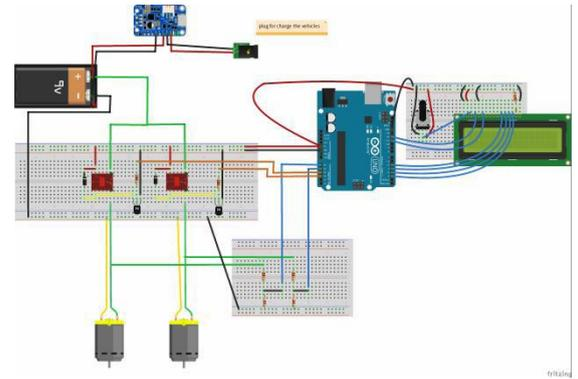
Figure 8: Circuit connection of demo project.
