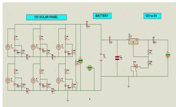
Figure 12: Solar panel charging circuit simulation.
