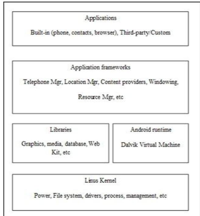
Fig. 1 Android Software layers
