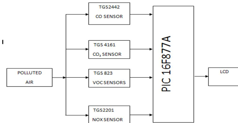
Fig. 2 Block Diagram of the Proposed System
