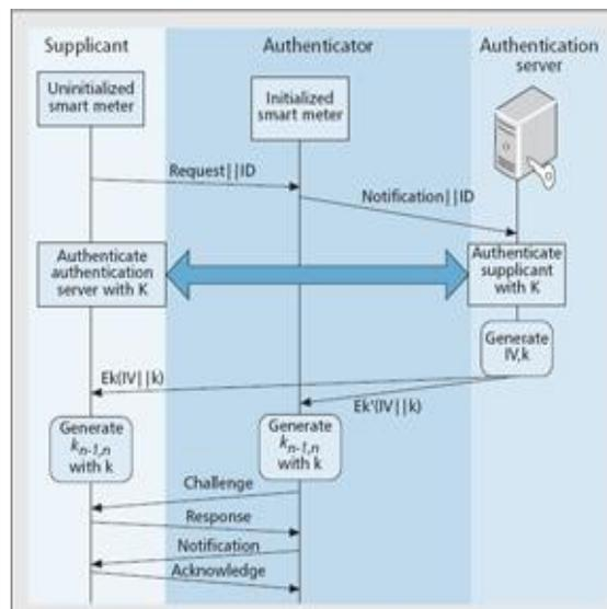
Fig.4. Initialization process and authentication
