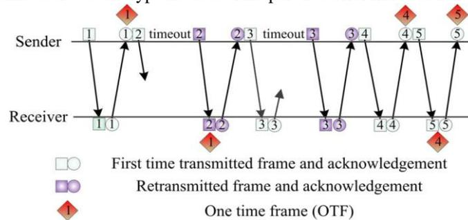
Fig.2. SW protocol and OTF identification
