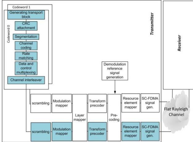
Fig. 1: LTE advanced system Model
