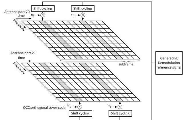
Fig. 2: Design of pilot pattern in a (2×2) MIMO SC-OFDM.
