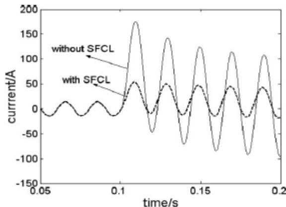
Fig.4: The fault current characteristics waveform (mode 1).
