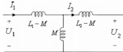
Fig.2: The equivalent circuit of the air-core superconducting transformer.
