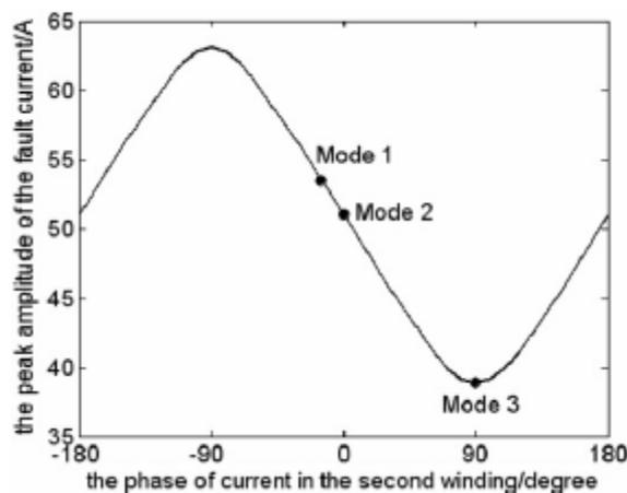
Fig. 8: The relationship between the peak amplitude of the fault current and the amplitude of  $I_b$  when the amplitude is constant.
