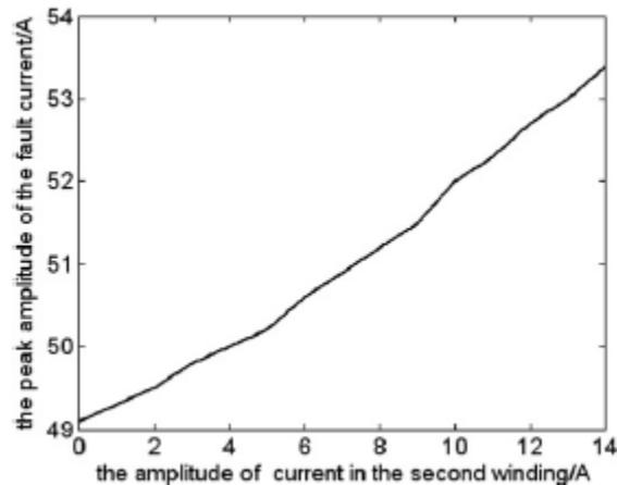
Fig. 7: The relationship between the peak amplitude of the fault current and the amplitude of  $I_b$  when the phase is constant.
