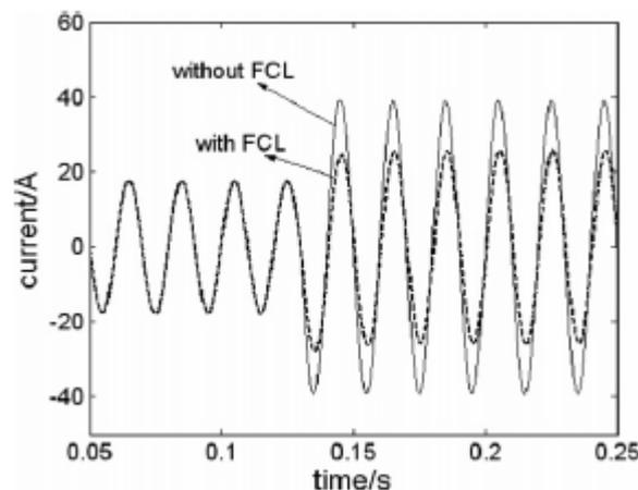
Fig.10: Fault current characteristics waveforms.
