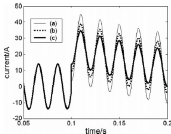
Fig.6: The fault current characteristics comparison under different amplitude
