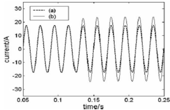
Fig.11: The characteristics of current for the second winding according to:(a) normal state and (b) fault state.
