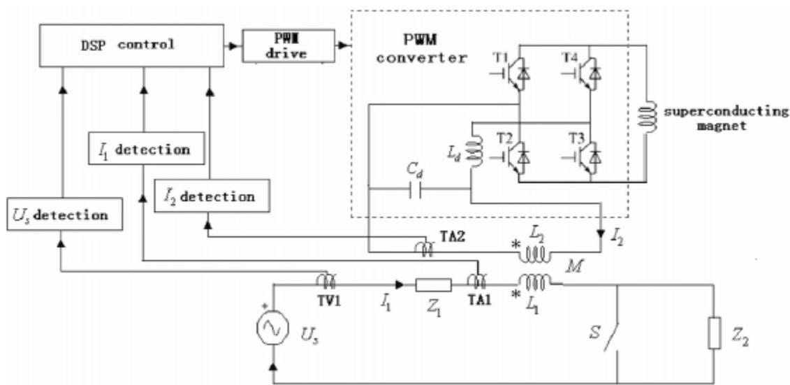
Fig.1: circuit arrangement of the active SFCL
