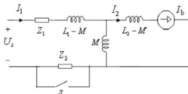
Fig.3: Active SFCL equivalent circuit
