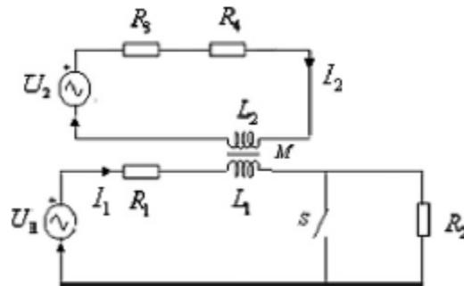
Fig.9: Experimental circuit of the FCL.  $L_1 = 5.98$  mH;  $L_2 = 5.92$  mH;  $M = 5.87$  mH;  $R_1 = R_3 = 0.6$   $\Omega$ ;  $R_2 = R_4 = 0.8$   $\Omega$ ;  $|\dot{U}_1| = |\dot{U}_2| = 25$  V.
