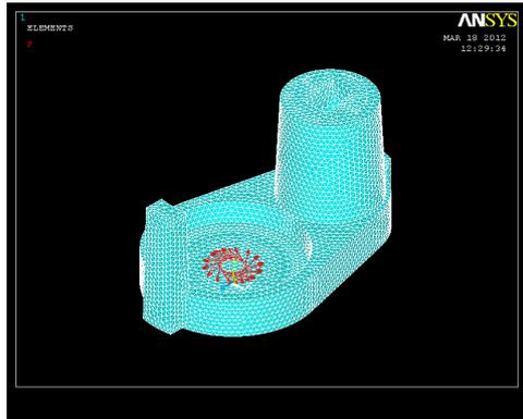
Figure-9: The meshed model with given force.
