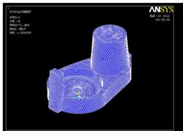
**Figure-16: Model for the frequency 71 Hertz**
