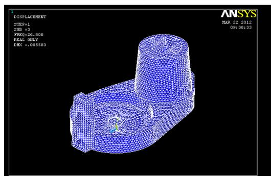
Figure -11: FE model for the frequency 26 Hertz Figure
