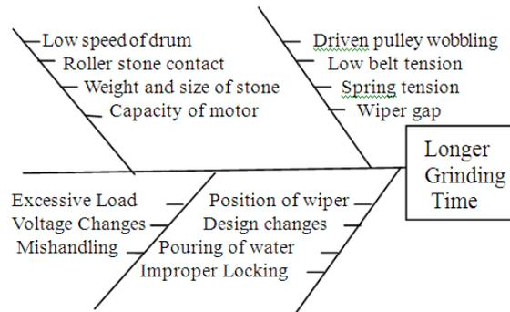
Figure 3.Cause and Effect Diagram
