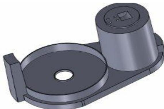
Figure 6.Three dimensional model of the wet grinder shell
