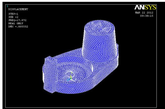
Figure-10: FE model for the frequency 17.87 Hertz
