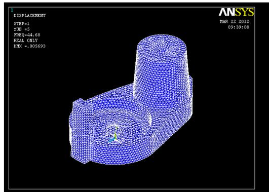
Figure-12: FE model for the frequency 35 Hertz Figure
