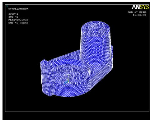
Figure -7: Meshed model of grinder shell
