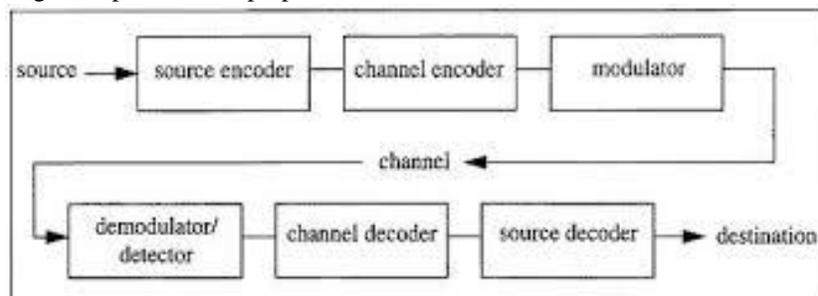
Figure 4 Block Diagram of Digital Communication
