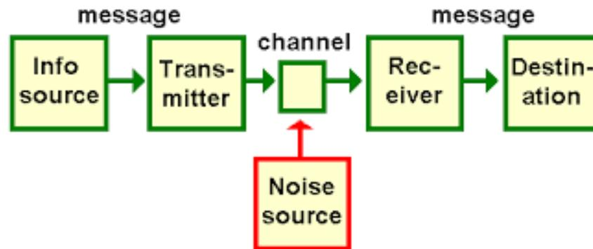
Figure 3 Block Diagram of Analog Communication
