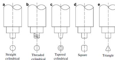
Fig. 5. FSW tool pin profiles.
