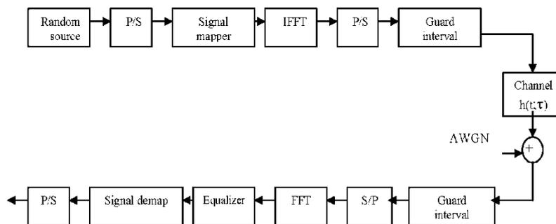
Fig.1 Block diagram of OFDM system
