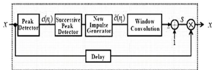
Fig 3: Peak windowing block in OFDM system
