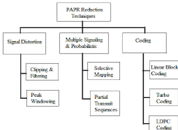
Fig. 2: Classification of PAPR reduction techniques
