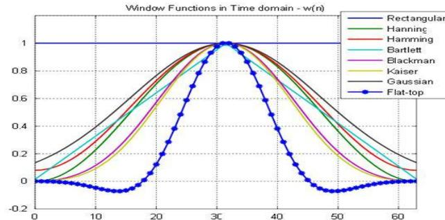
Fig 4: Different window functions in time domain
