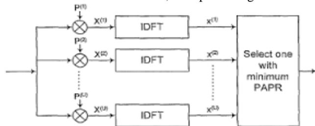
Fig 5: Block diagram of SLM technique [7]
