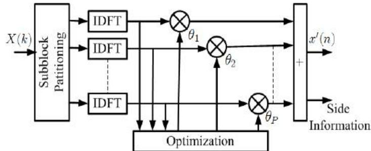
Fig. 6: Block Diagram of PTS Techniques [7]
