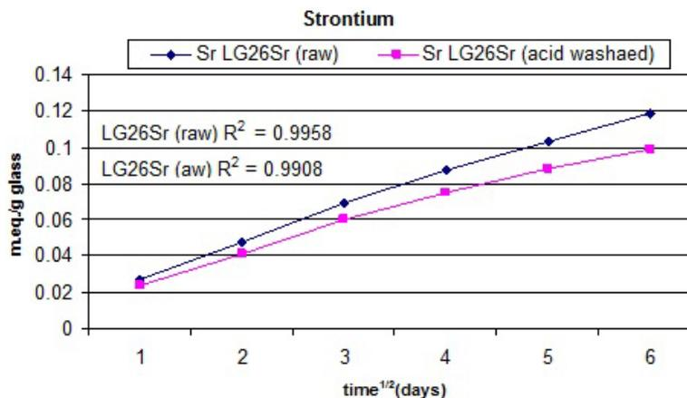
**Figure 3.** Cumulative release of strontium ions showing correlation coefficients for linear least squares fit.
