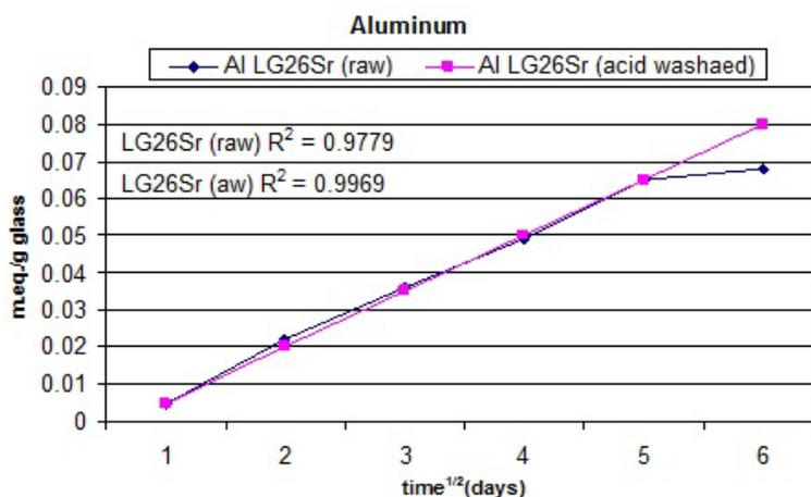
**Figure 2.** Cumulative release of aluminium ions showing correlation coefficients for linear least squares fit.
