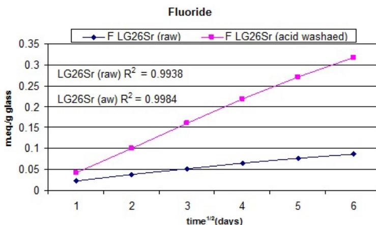
**Figure 1.** Cumulative release of fluoride ions into deionised water showing correlation coefficients for linear least squares fit.
