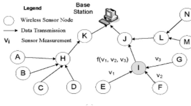
Fig. EXAMPLE OF AGGREGATION TREE
