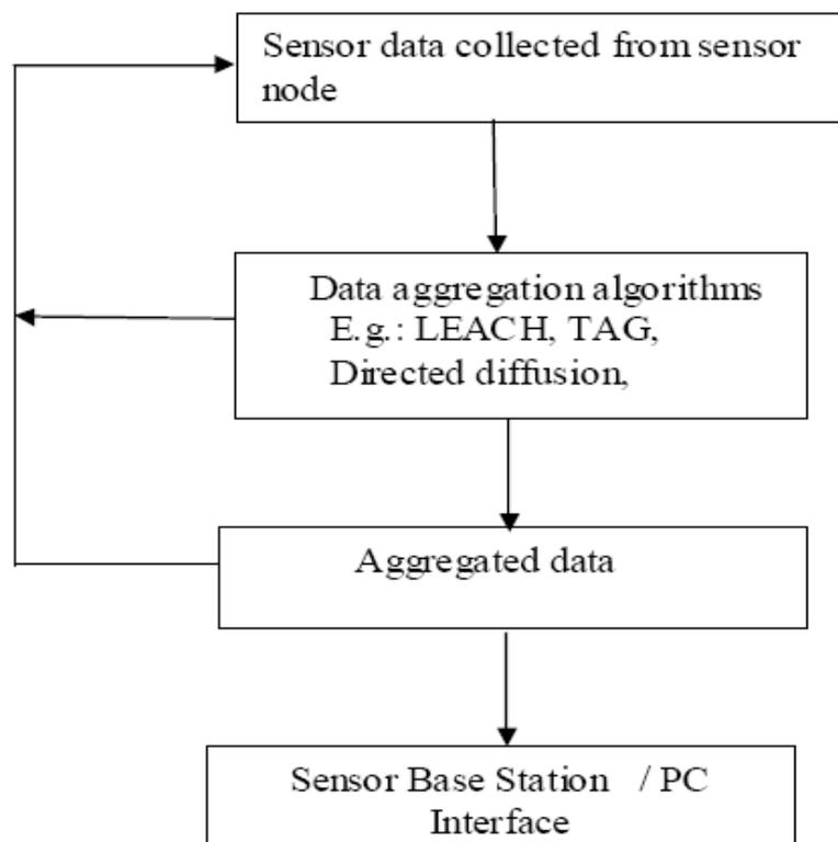
Fig. ARCHITECTURE OF DATA AGGREGATION
