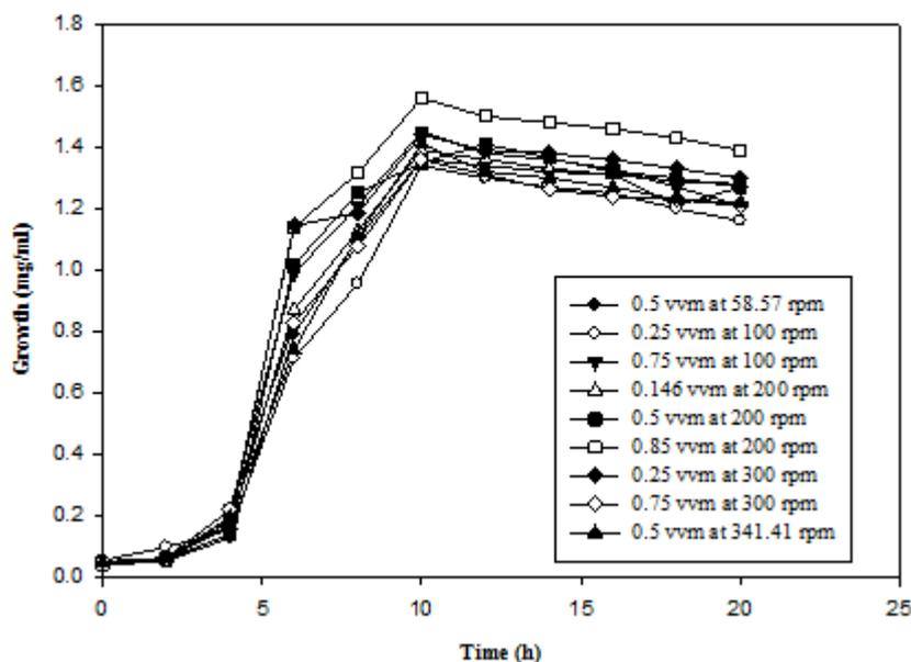
Figure 4a: Effect of agitation speed and aeration rate on cell mass production by *L. lactis* in fermenter.
