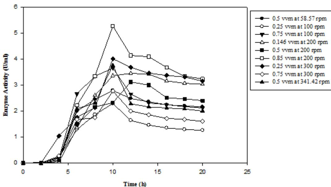
Figure 4b: Effect of agitation speed and aeration rate on dextranase activity of *L. lactis* in a laboratory fermenter.
