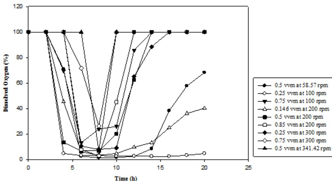
Figure 4c: Effect of agitation speed and aeration rate on dissolved oxygen during growth of *L. lactis* in laboratory fermenter.
