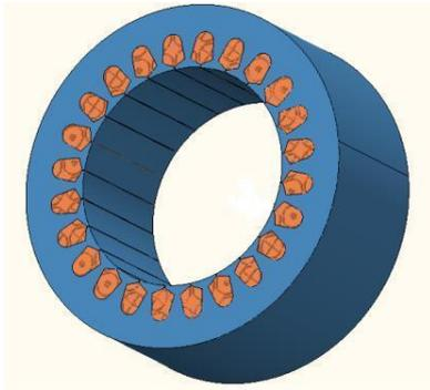
Fig. 1 Stator of IPM
