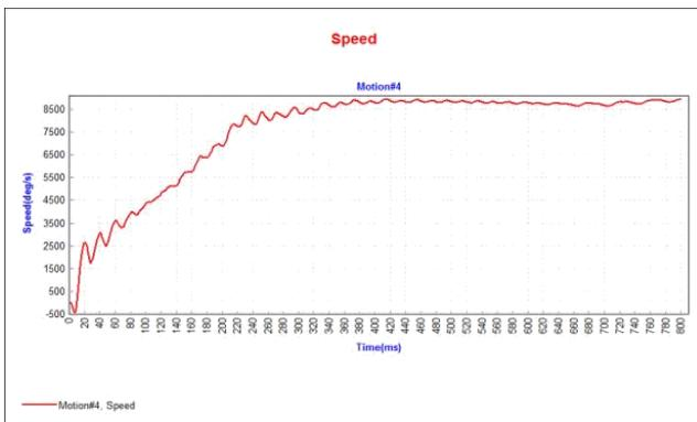
FIG. 7 (a) TORQUE, (b) SPEED CHARACTERISTICS OF IPMSM OF COMBINATION 4
