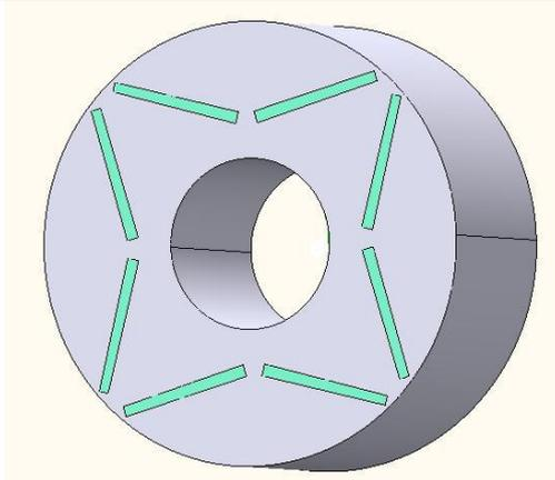
Fig. 2 IPM rotor
