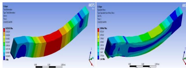
Fig.6.1.4 Total deformation and von-mises stress diagram of 10mm thick laminated wood
