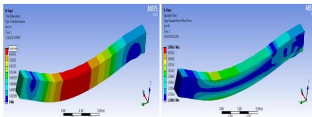
Fig.6.1.3 Total deformation and von-mises stress diagram of 15mm thick unjointed laminated wood
