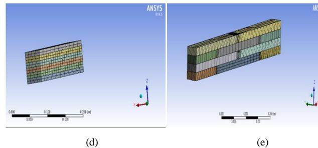
Fig.5.1.2 Meshed model (a) Solid wood(S) (b) Three layer laminated beam(A) (c) Four layer laminated beam (B) (d) Six layer laminated beam(C) (e) Jointed laminated wood with four layer having each lamina 15 mm thick(J)
