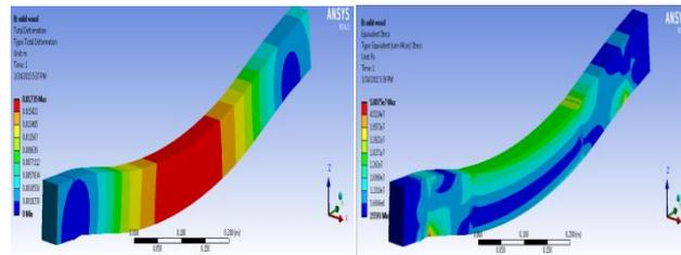
Fig.6.1.1 Total deformation and von-mises stress diagram of solid wood
