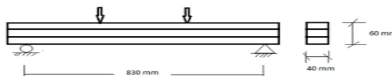
Fig. 5.1.1 Geometry of the model
