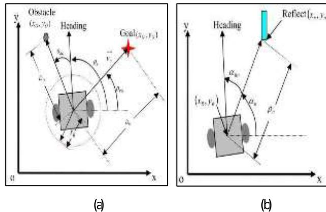
Figure 2. Localization by concurrent observation of several geometric beacons.
