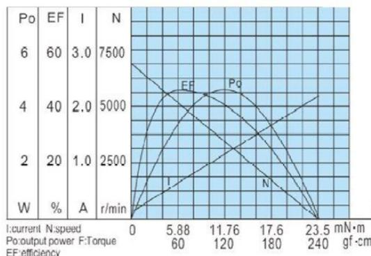
Figure 6. SPG30E-30K DC motor characteristics.
