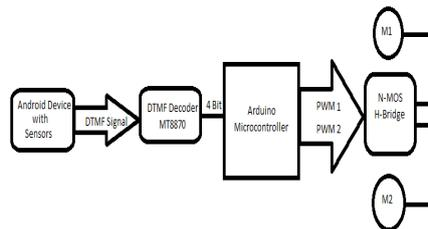
Figure 5. Robot motion block diagram.
