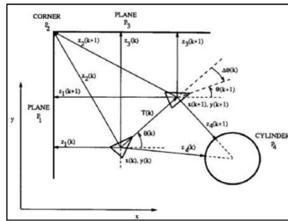
Figure 1. Localization by concurrent observation of several geometric beacons.
