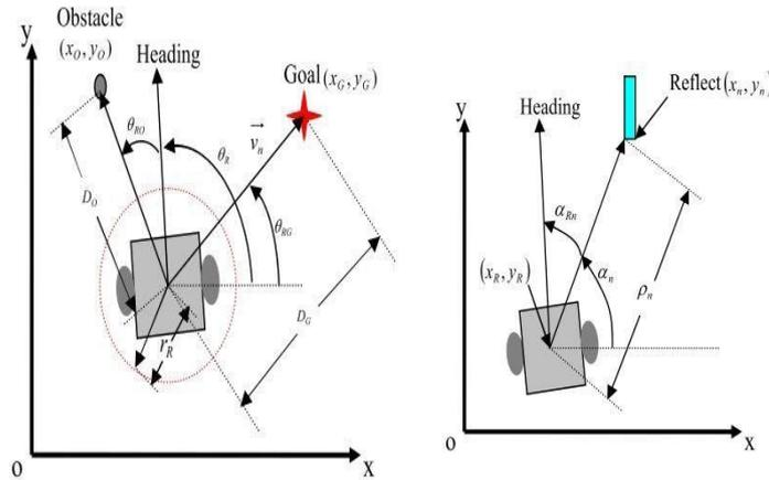
Figure 3. (a) Model of robot motion (b) model of location measurement.
