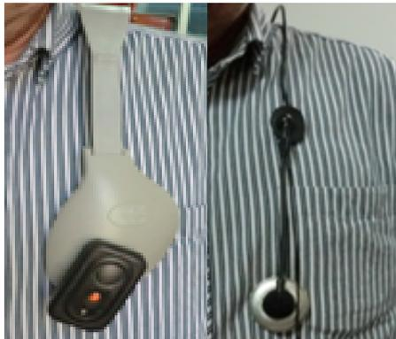
Figure 6. Shoulder belt type heart sounds collector.
