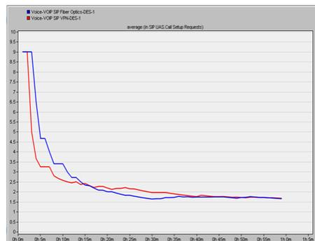
Figure 10: SIP UAS call setup requests.
