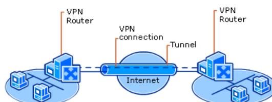
Figure 1: Tunneling path in the VPN.
