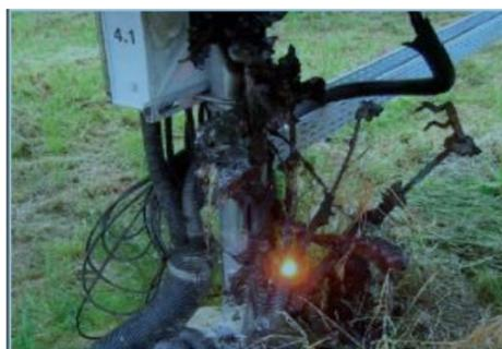
**Figure 3:** Arcing persists in the dc wiring even after a fire consumes a portion of the combiner box.
