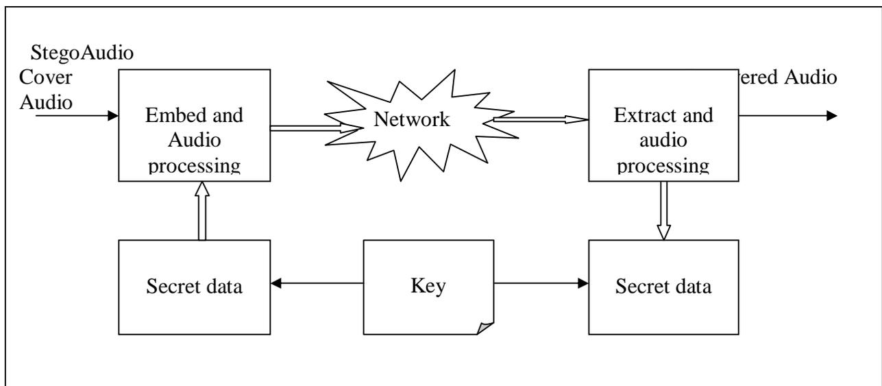
Fig no: 1.1 Block diagram for audio steganography
