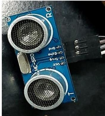
**Figure 1: Ultrasonic sensor.**
