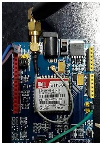
**Figure 2: GSM modem.**
