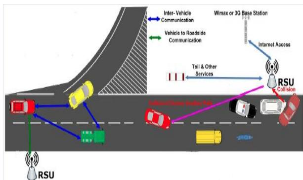
Fig. 1 VANET Data Exchange
