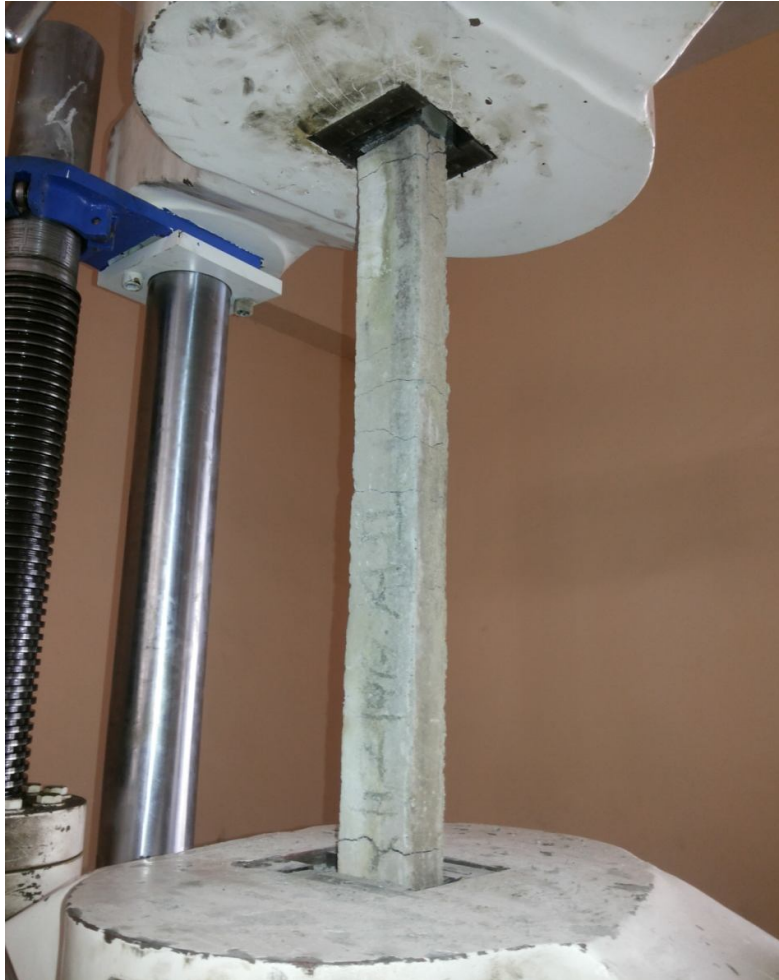
Figure 1: Typical Setup for Tensile test
