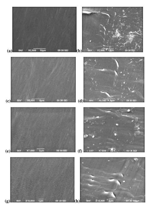
Fig.7 (a), (c), (e) and (g) untreated low density polyethylene at x2500, x5000, x7500 and x10000 respectively; (b), (d), (f) and (h) – low density polyethylene after 30 days incubation with Bacterial isolate 2 at x2500, x5000, x7500 and x10000 respectively.
