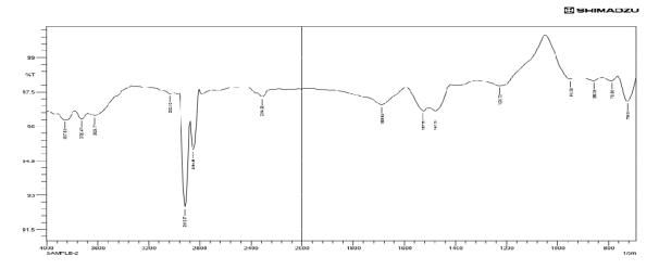
Fig.5 FTIR spectra of low density polyethylene after 30 days incubation with Bacterial isolate 2
