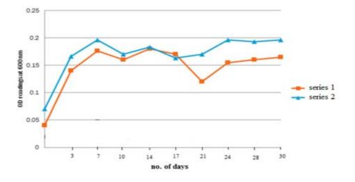
Fig 1 Growth curve of bacterial isolates during biodegradation assay
