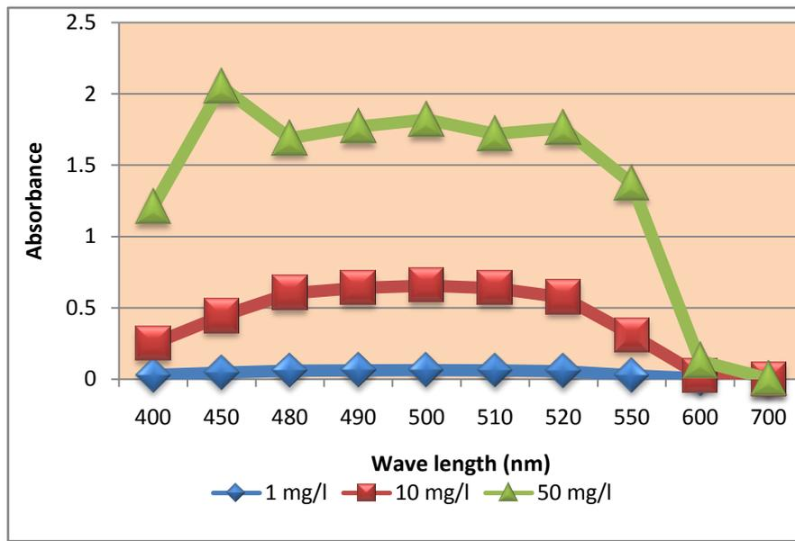
Fig. 3. Absorbance of Congo red solution versus the wavelength in the visible range (400 – 700 nm) at a pH of 7.6 for different concentrations
