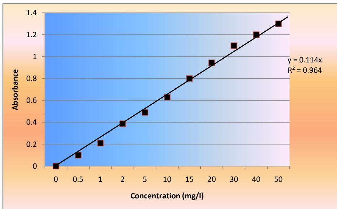
Fig. 5. Calibration plot for Congo Red at 500 nm
