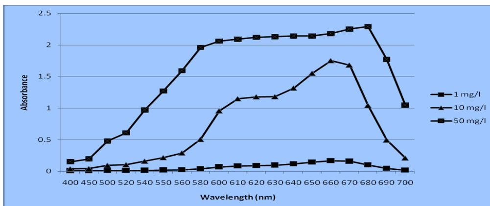
Fig. 2. Absorbance of Methylene Blue solution versus the wavelength in the visible range (400 – 700 nm) at a pH of 7.6 for different concentrations
