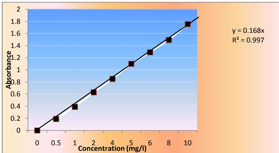
Fig. 4. Calibration plot for Methylene Blue at 660 nm
