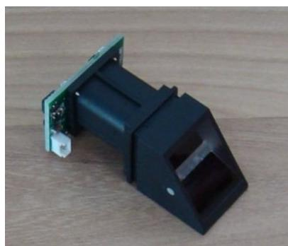
Fig. 4.R305 optical fingerprint scanner
