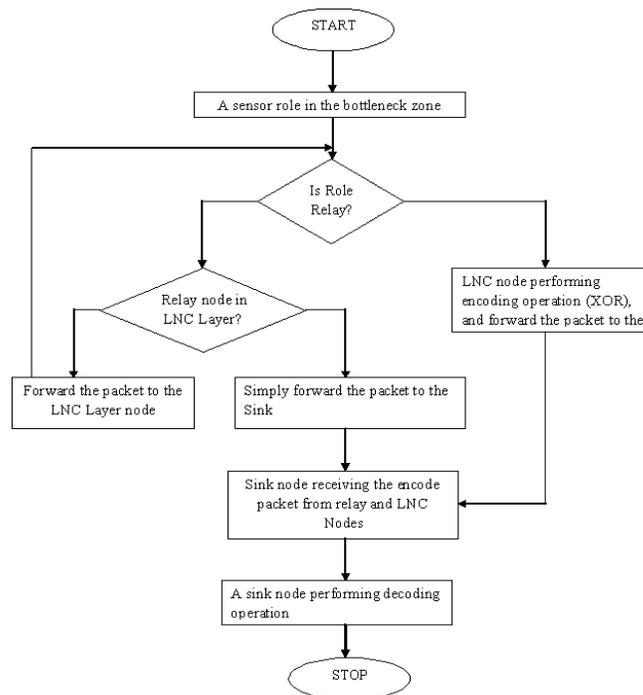
Fig 6: Flow chart of sensor node in bottleneck zone.
