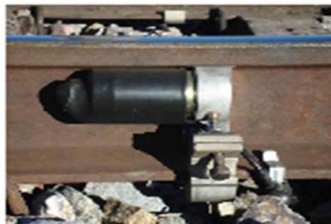
Fig.1 Ultrasonic Broken Rail Detector
