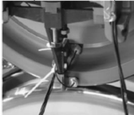
Fig.2 Model Figure to Fix the IR Sensor on the Wheel
