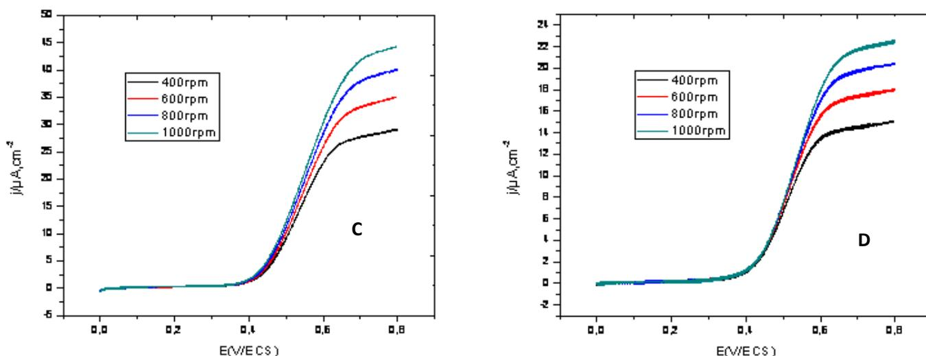
**Figure 3(C,D):** Polarogramme of 1 mM N'-Ferrocenylmethyl-N'-Phenylbenzohydrazide and 100 mM Bu<sub>4</sub>NBF<sub>4</sub> in CH<sub>2</sub>Cl<sub>2</sub> (A) at glassy carbon working electrode(B) at platinum working electrode, Pt counter electrode, and CSE reference electrode at 0.50 V.s<sup>-1</sup>. (Rotating rate 400, 600, 800, 1000 rpm).
