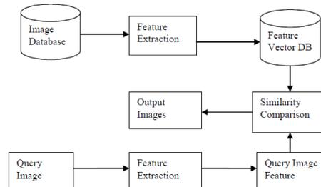
Figure 1: Block diagram for CBIR technique.
