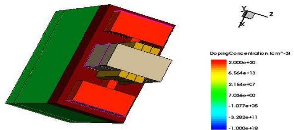
Fig -1(a) 3D Double or Tri-gate FinFET structure
