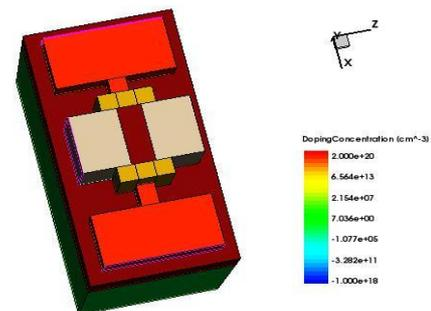
Fig-1(b) 3D Independent Gate FinFET structure
