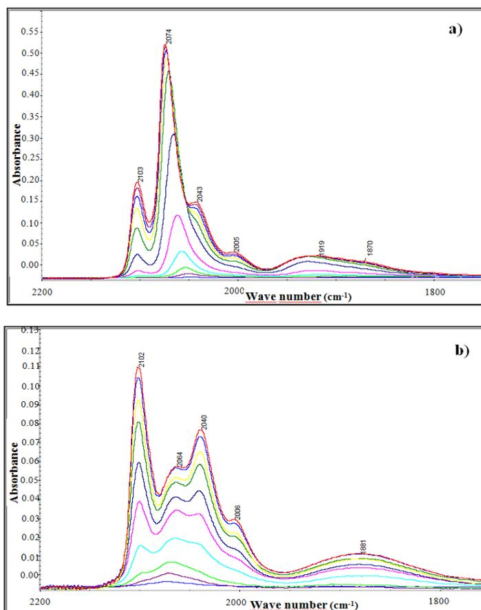
**Figure 1.** Spectra of adsorbed CO (with increasing CO amounts) on Rh/TiO<sub>2</sub> monometallic catalysts: a) parent sample, b) blank sample.
