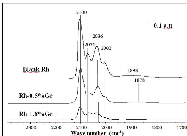
**Figure 2.** FTIR spectra of CO adsorbed on the Rh-based catalysts (blank and bimetallic Rh-X%Ge/TiO<sub>2</sub>).
