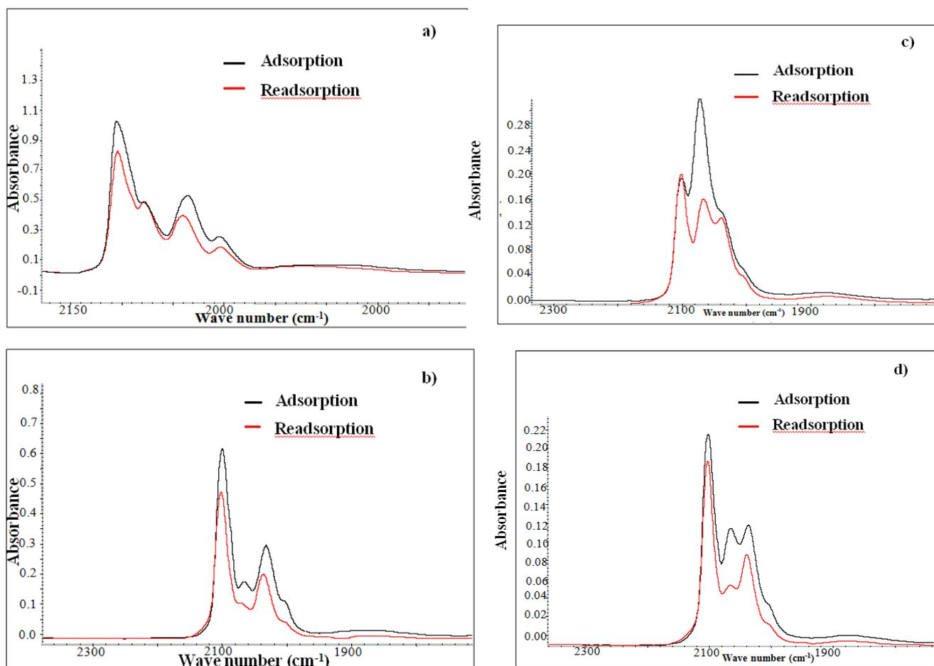
**Figure 4.** Spectra of CO adsorption and re-adsorption followed by FTIR on the Rh-X%Ge/TiO<sub>2</sub> catalysts: a) X=0 (blank sample), b) X=0.5, c) X=1.6, d) X=1.8.
