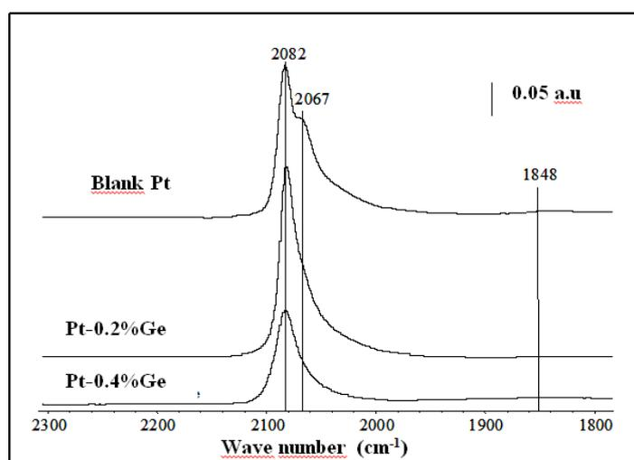
**Figure 3.** FTIR spectra of CO adsorbed on the Pt-based catalysts (blank and bimetallic Pt-X%Ge/TiO<sub>2</sub>).
