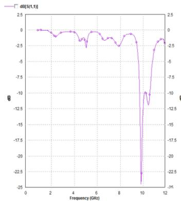
Fig. 2 (a) Return Loss Curve of Circular Patch
