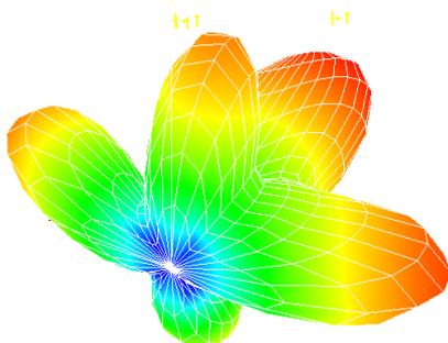
Fig. 2 (c) Gain Pattern of Circular Patch
