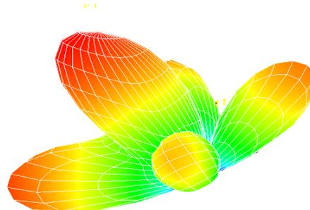
Fig. 2 (b) Directivity Pattern of Circular Patch
