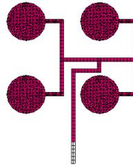
Fig. 1 (b) Circular Patch Antenna Array
