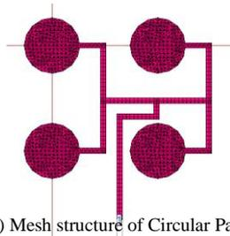
Fig. 1(c) Mesh structure of Circular Patch
